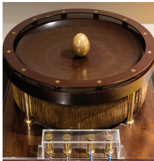
Photo 2: Induction motor with Egg shaped rotor.
